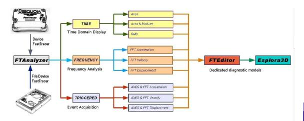
FTAnalyzer: measurements and diagnostics
