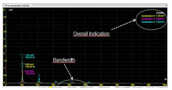
Once the *bandwidth* is defined (between MinX(Hz) and MaxX(Hz)) the Overall is computed according to the following formula
