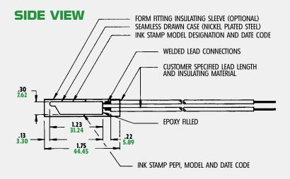
A snap-action thermostat/thermal protector with the highest contact ratings of any of our controls. Suitable for use on 120/240 VAC loads. Available with variety of bi-metallic elements to enhance performance characteristics.
