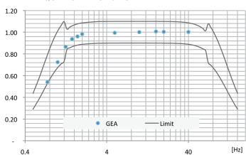
Test performed at INRIM, primary Italian laboratory for calibration. Limit curve as per DIN 45669-1
