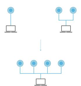
With **TRADITIONAL HANDHELD SYSTEM** or **VIBROMETER** the entire measurement chain need to be duplicated. Furthermore, managing several system at the same time require dedicated cabling.
