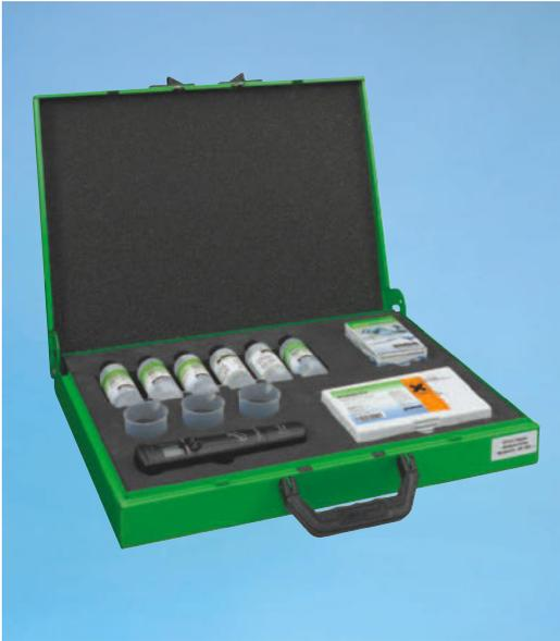
GENO-therm® analysis case including molybdenum test kit
