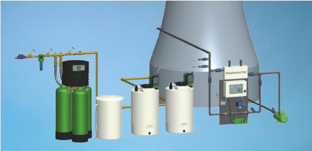
Installation example for cooling water treatment systems
